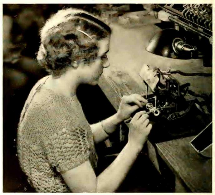
NE of the most delicate processes in Sylvania tube manufacture is "mount assembly"—a job that demands exceptional precision and skill. For each tube part must be accurately spaced in relation to other elements . . . and carefully welded in place.
